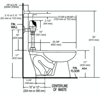
When installing the Sloan SOLIS<sup>®</sup> in a handicap stall: Per the ADA Guidelines (section 604.9.4) it is recommended that the grab bars be split or shifted to the wide side of the stall.
